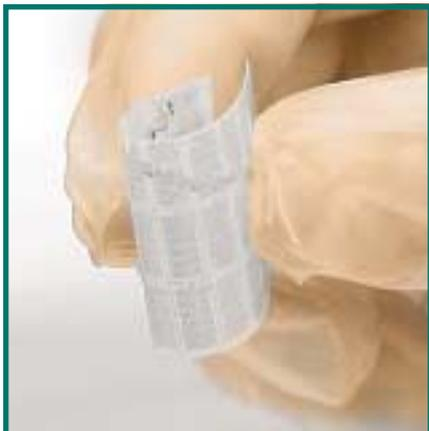
*NanoHorizons high-performance polycrystalline thin film transistors on a flexible polymer*
